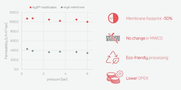
Ecofriendly Hy2F® functionalization of an ultrafiltration PES membrane shows enhanced performance in permeation over a pressure range from 0.5 to 6 bar in comparison to the unmodified membrane. The membrane's structure, molecular-weight cut-off and fouling tendency remain unaffected.
